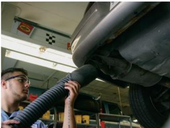
FIGURE 9–31 Whenever a vehicle is in a stall with the engine running, connect a shop exhaust hose(s) to the tail pipe
