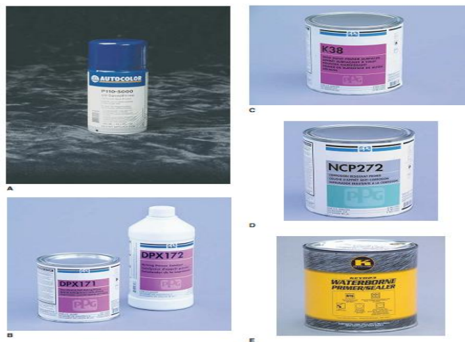
Figure (A) Plain primer is handy for rapidly priming small repair areas when the area is very smooth and ready for paint. (B) Etching primer is applied to bare metal. It contains acid that will eat into and bond to sheet metal. (C) High-build primer-surfacer is a very thick primer and is ideal for spraying over body filler repair areas. It will build up quickly
